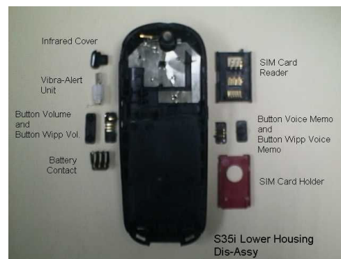
PHOTO 2.10 Disassembly Lower Housing – STEP 2
